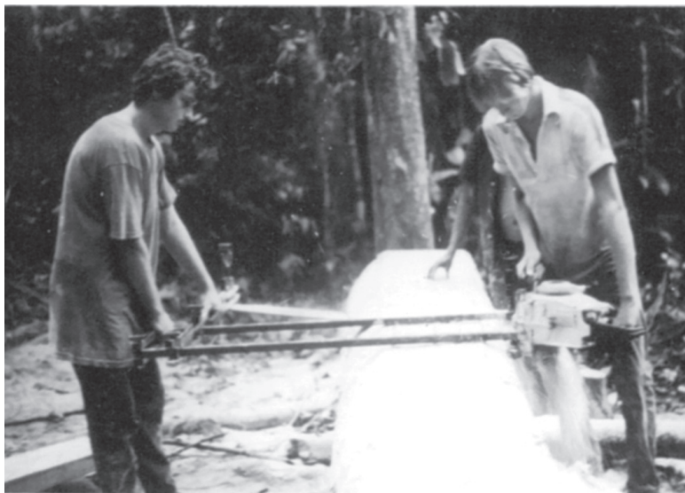
Cutting lumber with chainsaw mill, 1980
